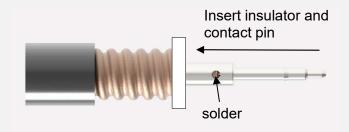
3.) Rewind the cable with the solder wire (dia.: 1,0mm / length: 105mm)
